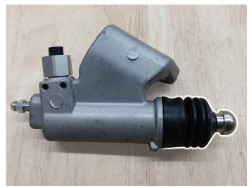
Note: Use a light coat of grease/oil when installing the Pushrod.
